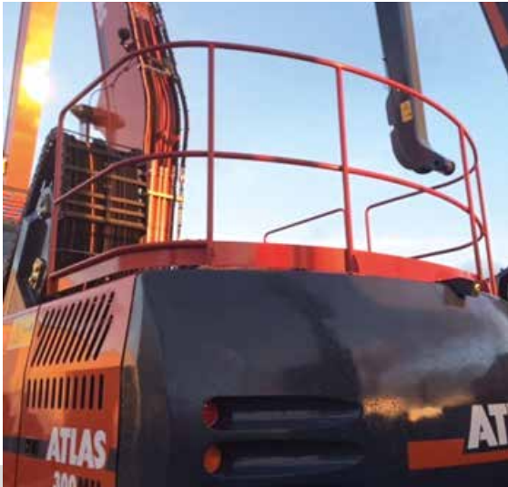
HANDRAIL FOR SUPERSTRUCTURE
