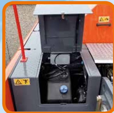
Easily accessible AdBlue® tank
