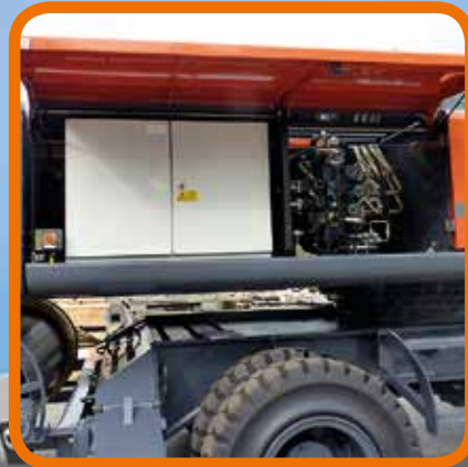
Control cabinet for E-Drive
