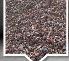
Rubble, asphalt, tiles, bricks, natural Final particle size is 0-60 mm at a throughput rate of 80-100 t/h (concrete) and 160-200 t/h (C&D waste).
