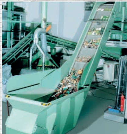
Pre-crushing of electronics wastes (printed circuit boards)
