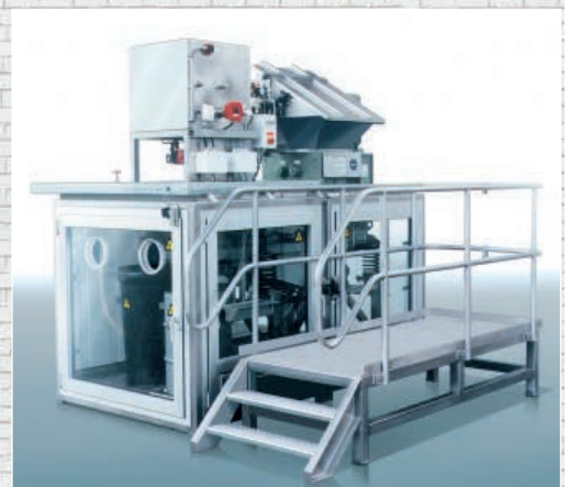
Volume reduce of low-level radioactive materials
