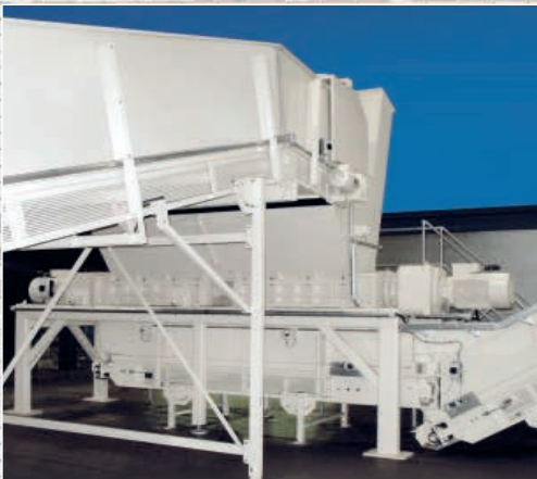
Twin-type shredder unit for the destruction of reject material
