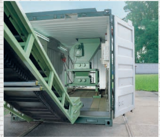
Movable container with integrated two-stage crusher for the shredding of plastic containers
