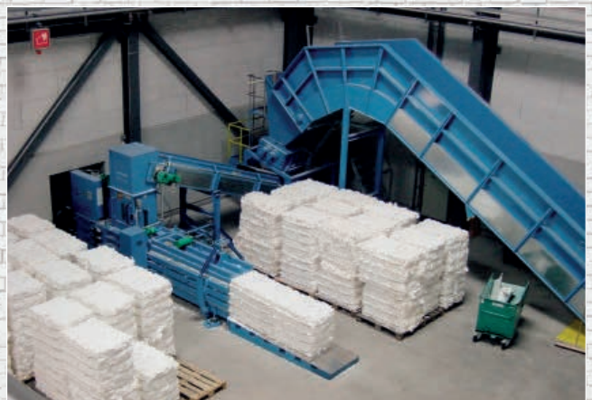
Shredder with baler for discharging production residues
