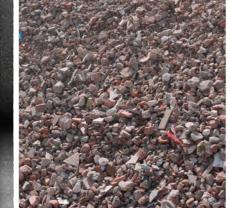
Final particle size is 0-55 mm at a throughput rate up to 95 t/h in conre-(shortest side not larger than 500 mm). te and up to 110 t/h in C&D waste.
