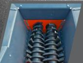
Large-sized crushing unit – therefore less preparation necessary with e.g. concrete shears and resistant against larger metal parts.
