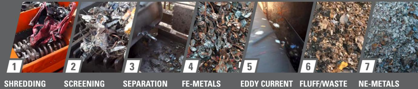
1 SHREDDING 2 SCREENING 3 SEPARATION 4 FE-METALS 5 EDDY CURRENT 6 FLUFF/WASTE 7 NE-METALS
